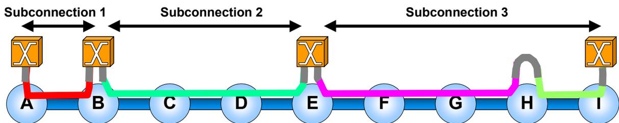
**Figure 5** Subconnections remain in the all-optical layer except for the endpoints, where they enter the O-E-O layer. Three subconnections are illustrated in the figure. Subconnection 1 extends over a single hop. Subconnection 2 optically bypasses Nodes C and D. Subconnection 3 optically bypasses Nodes F and G; the regeneration at Node H is static; i.e., it does not utilize an O-E-O crossconnect.
