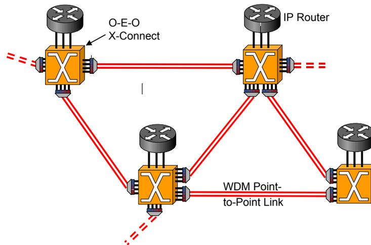
**Figure 1** The conventional IP-over-optical reference model, based on O-E-O crossconnects and WDM point-to-point links. The IP router layer is connected to the crossconnect layer.
