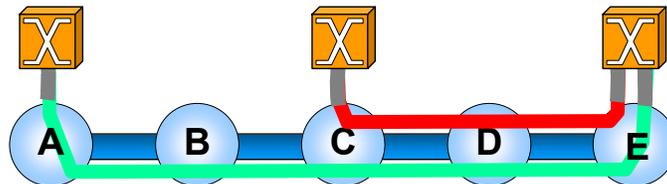
**Figure 6** The desired connection is from A to C, however, the only two existing subconnections are A to E and E to C. The O-E-O layer determines whether the cost of this path is within an acceptable threshold. If not, it can request that the all-optical layer establish more subconnections.
