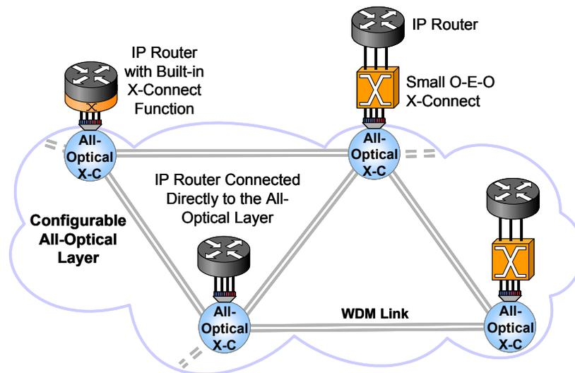
**Figure 2** The IP-over-optical reference model based on a configurable all-optical layer. A layer of small O-E-O crossconnects can exist over the all-optical layer. The IP router can be connected to an O-E-O crossconnect or directly to the all-optical layer. Some IP routers have a built-in crossconnect function.
