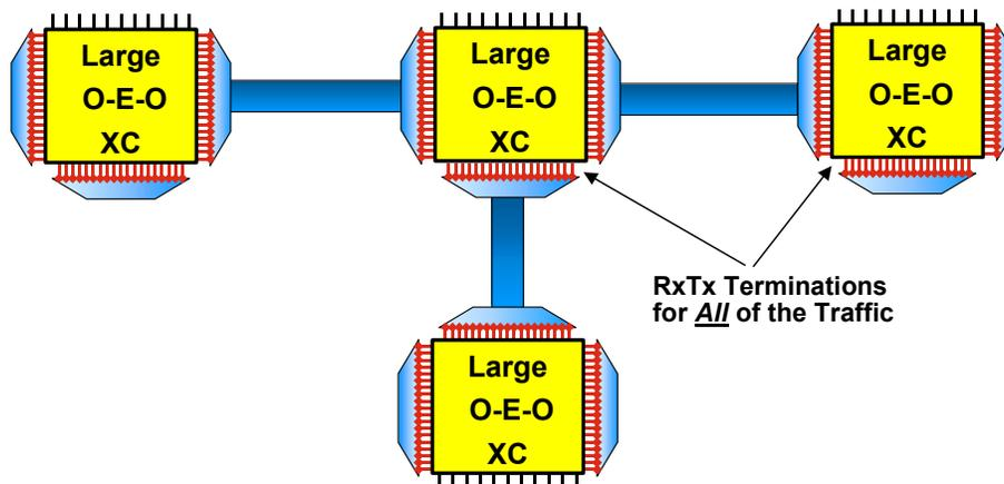
**Figure 3** In the conventional architecture, O-E-O crossconnects are interconnected by point-to-point WDM links. At each node, Tx/Rx line cards are needed for all of the traffic, regardless of whether it is express or local.
