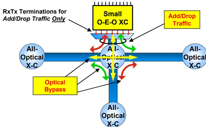
**Figure 4** In the all-optical architecture, ultra-long reach is combined with all-optical switches such that Tx/Rx line cards are required only for local add/drop traffic. The remaining wavelengths optically bypass the node.
