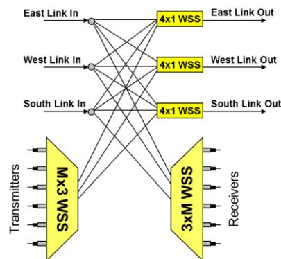
Figure 8. An M×N WSS is deployed to provide contentionless operation. Alternatively, an M×N MCS can be used.
