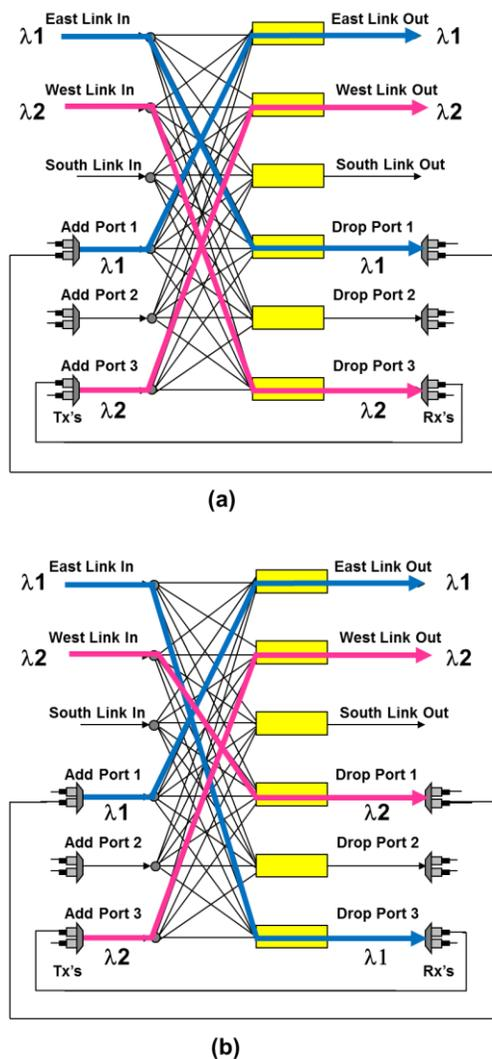
Figure 5. Shared restoration where pre-lit segments are concatenated to form the restoration path. Two pre-lit segments are shown, one on  $\lambda_1$  and one on  $\lambda_2$ . (a) The configuration prior to failure. (b) The desired configuration after a failure occurs, where the  $\lambda_1$  segment must be concatenated to the  $\lambda_2$  segment. To support this operation,  $\lambda_2$  must be available on drop port 1 and  $\lambda_1$  must be available on drop port 3.
