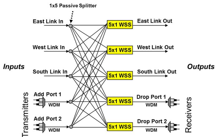
Figure 1. A broadcast & select ROADM with three network input/output fiber pairs and two add/drop ports. The ROADM inputs are on the left; the outputs are on the right. If it is desired that three connections, all routed on  $\lambda_1$ , be sourced/terminated at this node, then one of these connections will be blocked due to wavelength contention on the add/drop ports.
