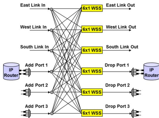
Figure 2. An IP router, which interfaces to add/drop port 1, wants to establish a connection on the East and West links. If  $\lambda_1$  is the only available wavelength on both of these links, then one of the connections will be blocked due to wavelength contention on the add/drop port.
