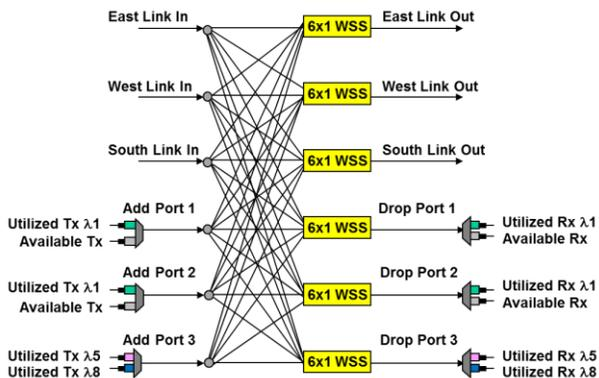
Figure 7. Assume that a new connection is desired on  $\lambda_1$ . The only available transponders (Tx/Rx's) are located on add/drop ports 1 and 2. However, the only add/drop port with  $\lambda_1$  available is port 3. Thus, the new connection would be blocked.
