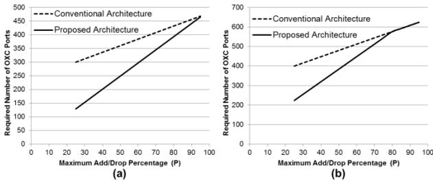
**Fig. 3** Savings in port size provided by the proposed architecture for: (a) A typical core node, with degree 3 and 80 wavelengths per fiber; and (b) A typical metro junction-node, with degree 8 and 40 wavelengths per fiber.
