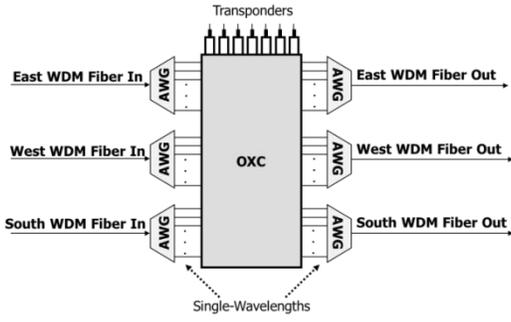
**Fig. 1** A WS CDC ROADM. In the configuration shown, the OXC switches single-wavelength signals.
