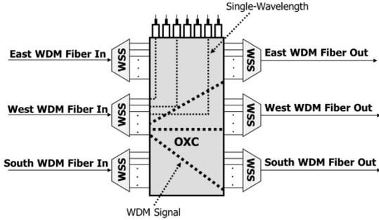
**Fig. 2** WSSs are used for the mux/demux in this WS CDC ROADM. Potential connectivity from the West input fiber is shown. Thick dotted lines indicate a WDM signal; thin dotted lines carry a single wavelength.
