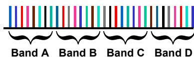
Fig. 9. In this example of wavelength banding, the 32 wavelengths in the spectral comb are partitioned into 4 bands, each composed of 8 contiguous wavelengths. In general, only a subset of the bands needs to be dropped at each node.
